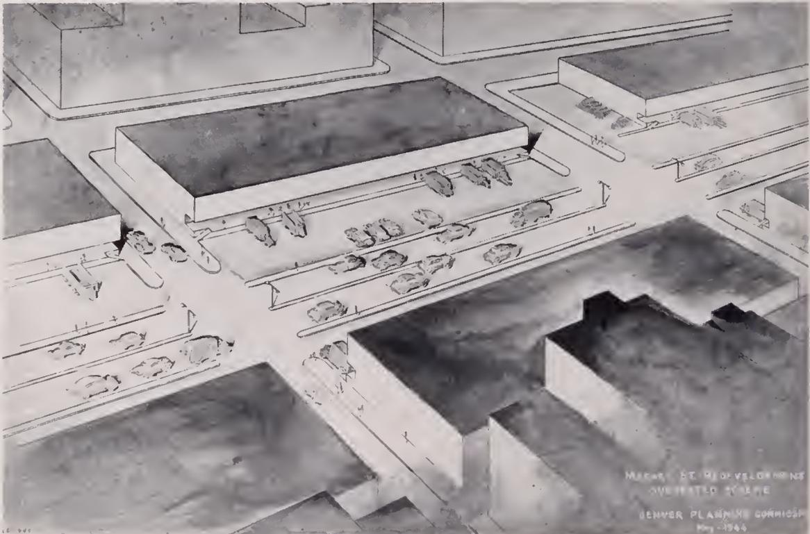
FIG. 17—The city's proposed Market Street improvement would provide wide loading zones for trucks.
