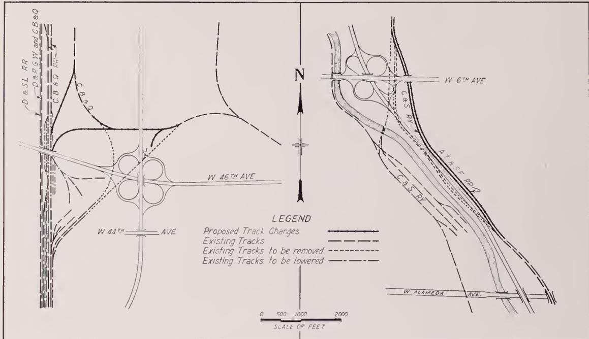
FIG. 28—Two major railroad track changes proposed to simplify construction of the Valley Highway.
