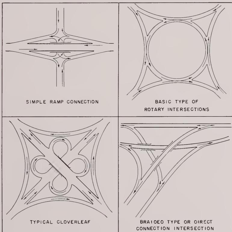
FIG. 21—Some types of traffic interchange, represented diagrammatically.
