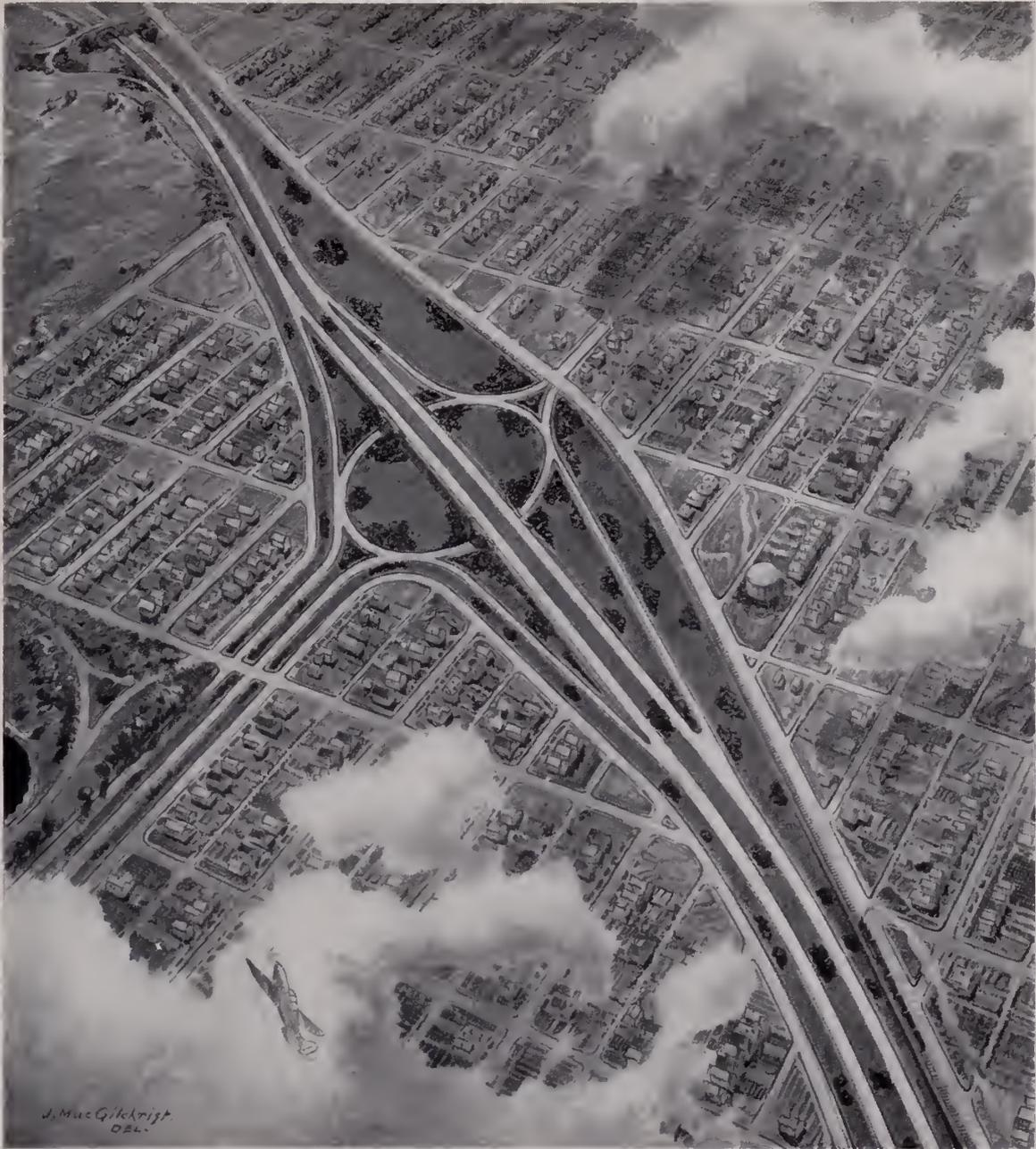
FIG. 25—How the Downing Street rotary will appear. The branch line of the Colorado & Southern along Buchtel Boulevard is at the right-hand edge of the highway right of way. Downing Street to the left of the Valley Highway is shown as it will be when widened.
