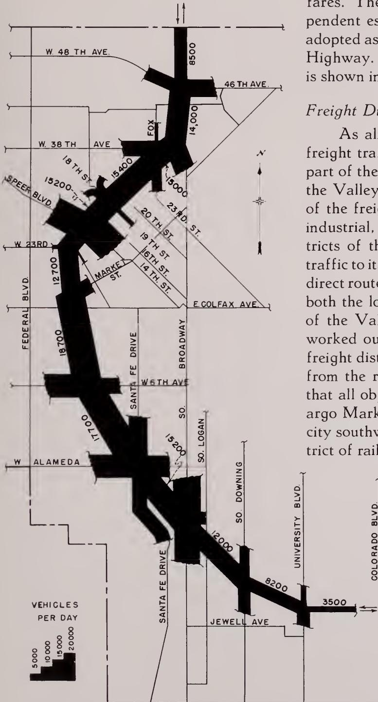
FIG. 18—Flow chart of the initial traffic on the Valley Highway as forecast from traffic counts.
