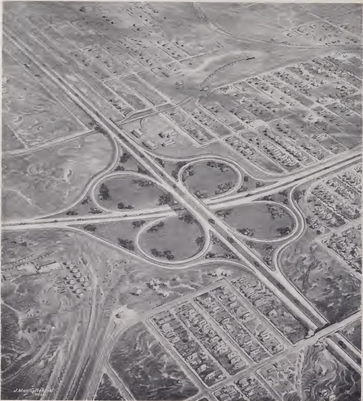
FIG. 23—Sketch of the projected 46th Avenue cloverleaf of the Valley Highway, seen looking northeast; at the right is the connection to East 46th Avenue, at the left curve to join 48th Avenue.
